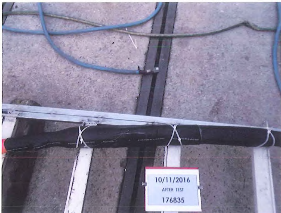
Photo 14: after thermal short-circuit tests on screen/ armour (nr. 176835)
