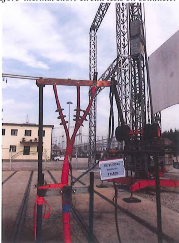
Photo 4: before thermal short-circuit tests on conductor (nr. 176828)
