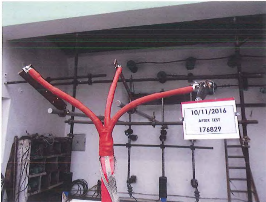
Photo 5: after thermal short-circuit tests on conductor (nr. 176829)
