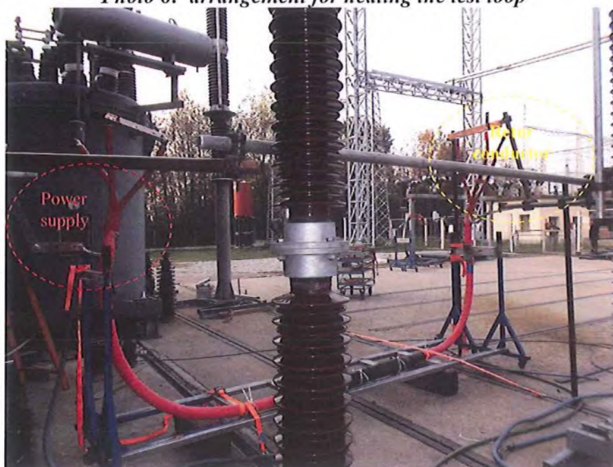
Photo 9: arrangement for test on screen/armor
