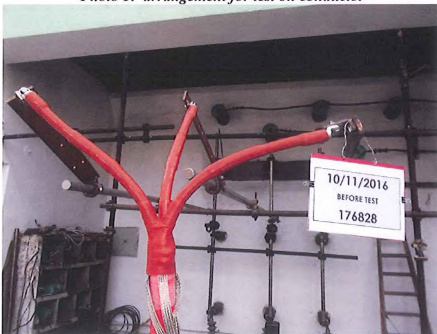
Photo 2: before thermal short-circuit tests on conductor (nr. 176828)
