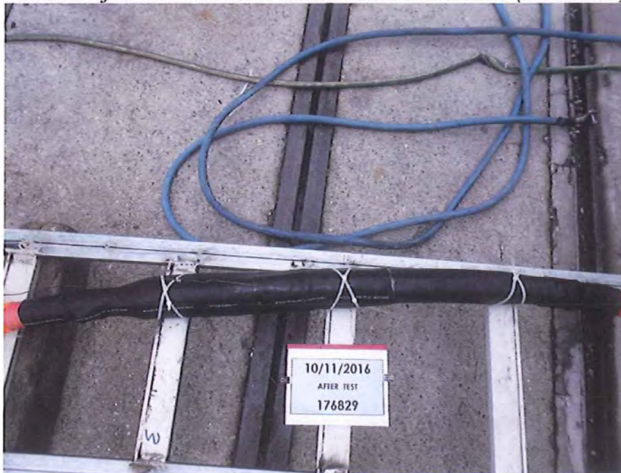
Photo 6: after thermal short-circuit tests on conductor (nr. 176829)
