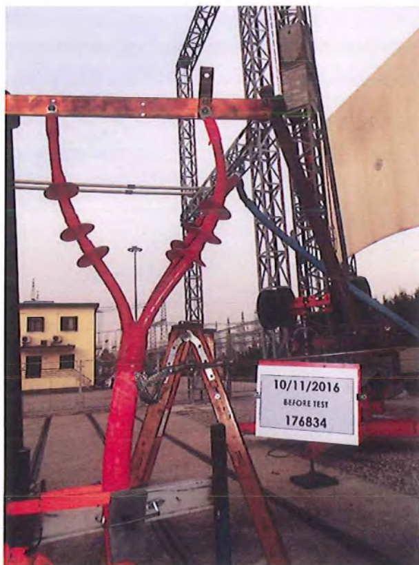
Photo 12: before thermal short-circuit tests on screen/armour (nr. 176834)
