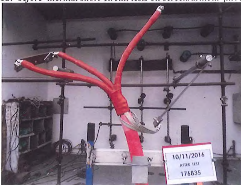
Photo 13: after thermal short-circuit tests on screen/armour (nr. 176835)
