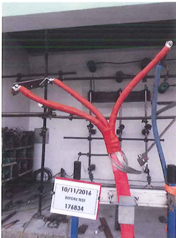
Photo 10: before thermal short-circuit tests on screen/armour (nr. 176834)
